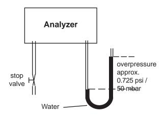
Fig. 7-1: Leak Testing With U-Turn Manometer
